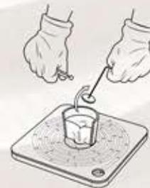
**3.** At a specified temperature pull the plug and the metal will drain down a spiral.
