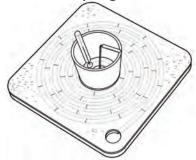
Full fill the cup with the melt metal. Pour the metal directly inside the cup and do not touch or move the cup to avoid leaking of the metal. Do not over-fill the cup so the metal will flow over the measuring scale.
